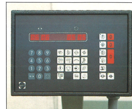
Clear, distinct design: control desk with sheet-covered keyboard and digital display.
