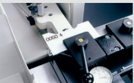
**Profile ground knives** are shaped and resharpened to a profile template on the back of the knife. This ensures absolute profile precision and optimum cutting angles for all types of species and materials. Sharp tools, perfectly ground for precision running.
