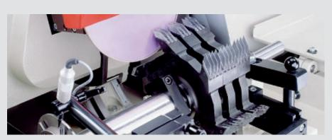
Mill-to-pattern cutter heads are sharpened at the face. Individually or a set – you always achieve maximum precision with the Rondamat. Mill-to-pattern tools are used for making special parts such as dowels, grooves, and profiles for edge gluing.
