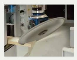
The sawing system enabled a multitude of processings (e.g. compound angles, birds mouth, longitudinal cuts).
