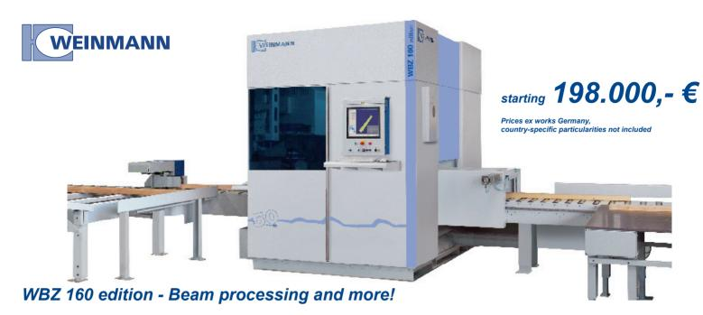
The beam processing station WBZ 160 editon was designed for the production of wall panels, trusses and beam processing. Its modular structure enables it to be tailored to your specific requirements. Weinmann offers the WBZ 160 edition with complete tool equipment incl. dove tail router, marking and labeling system as well as a extensive software packages at a very favourable jubilee price.
