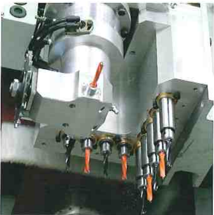
■ The boring unit is equipped with 9 vert. Spindles. Grooving saw + hor. drills unit is available as option
