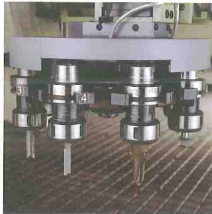
■ The automatic tool change provide a 8 position tool carousel
