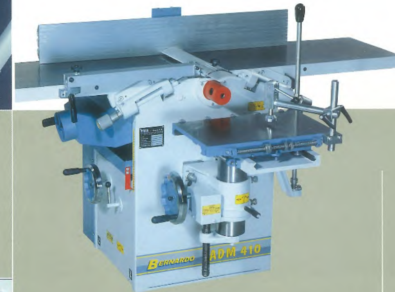
ADM 410 with mortiser, ideal option for slotting and mortising.
