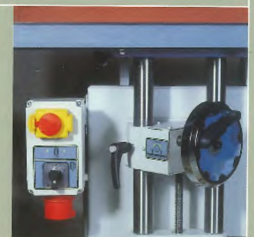
Handwheel for table height adjustment with clamping possibility and electric control box.
