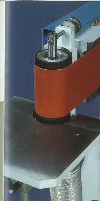
Adjustable supporting table with dust collection and rubber coated sanding roller for sanding of curved workpieces.
