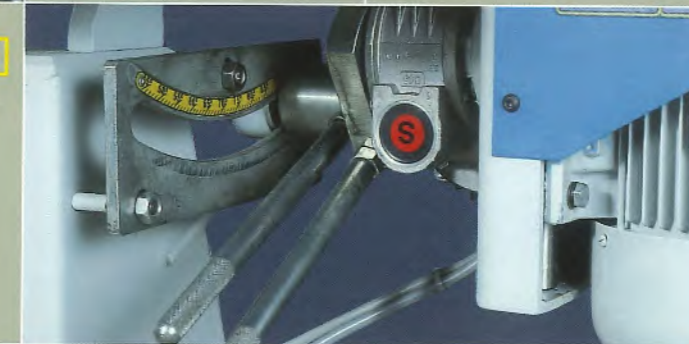
Sanding oscillation with separate motor and lever for tilting of the aggregate with scale.
