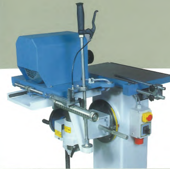
LBM 200 with mounted 4-size rotor group with fixed positions at 16-22-25-32 mm.
