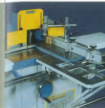
T 800 i for tenoning with front sided carriage, tenoning table and extraction hood.
