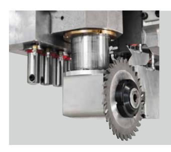
For cutting, a dedicated blade unit can be fitted, either in a fixed position or with adjustable angle 0-90°.
