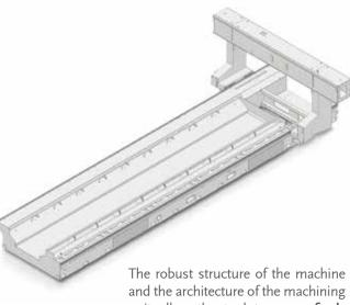
The robust structure of the machine and the architecture of the machining unit allow the tool to move freely around parts of complex shape, and perform three-dimensional machining with high precision and maximum finish quality.
