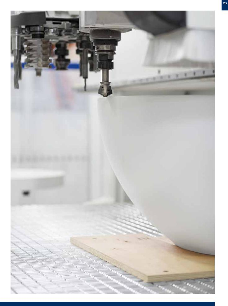
Prisma 5-axis machining unit
