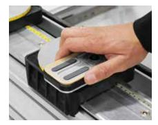
The quick coupling and "tubeless" vacuum transmission system make the worktable freely configurable depending on the geometries of the work pieces to be machined.
