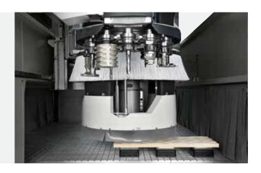
While routing with the tool in vertical position, it is utilized the **inner hood**, which is more effective for this kind of operations, thanks to its reduced dimensions.
