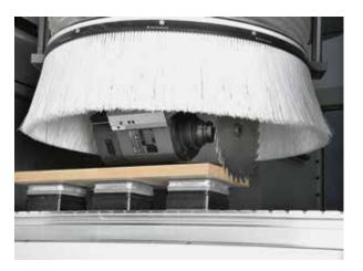
During 5-axis routing, it is utilized the **outer hood**, which has adequate dimensions to cover all tool movements.
