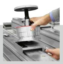
Switching from suction cups to clamps and vice versa is quick and easy. The quick coupling developed by SCM allows operators to change the accessory at the press of a button.
