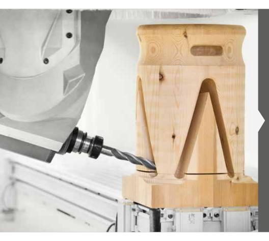
It is possible to process work pieces with 500 mm working height, on both upper side and lateral sides, thanks to the high Z-axis vertical stroke.
