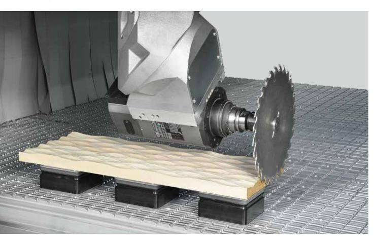
The electrospindle, designed and manufactured by SCM, develops an output of 17 kW and reaches maximum rotation speed of 24000 rpm. Excellent performances making the machine optimal both for routing with heavy stock removal and profiling at high rotation speed.
