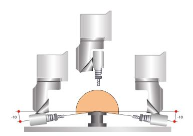
Prisma machining unit geometry allows it to operate at **angles of up to 10**° below the work piece supporting surface.
