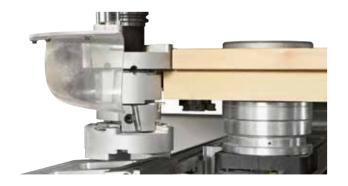
The **TTS** (**Total Torque System**), unique to SCM, mechanically locks the rotating axis during machining with tools in vertical position, increasing system stiffness.
