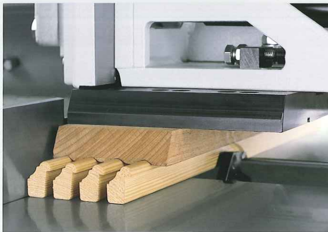
Adapter plate when using replaceable counter profiles. Control of profiles with great differences in height within a profile. This means that workpieces with complicated shapes are held securely for the best surface finish and tolerances. This is a great advantage for difficult to control profiles such as dowels: high surface quality! No surface finish problems caused by movement when workpieces are separated.
