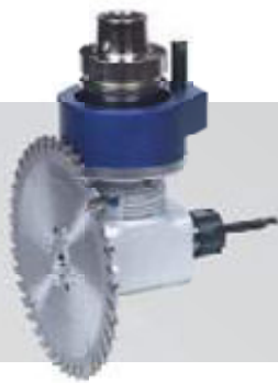
HSK F63 Dual angle head with 1 output for drill-, milling tool and 1 ER 25/WELDON output with screw mounted saw blade, max. Ø 180 mm Order no. 300-24-012
