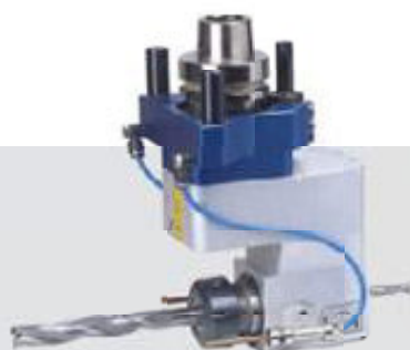
HSK F63 Lock recess aggregate with 2 ER 25 outputs for drilling or milling tooling and two compressed air dust removal jets Order no. 300-24-017
