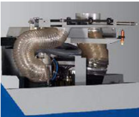
Program controlled extraction connection Ensures an efficient extraction result.
