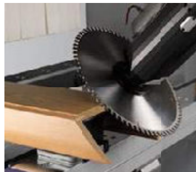
Door frame manufacturing
