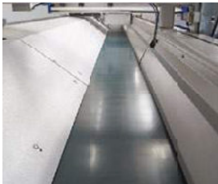
Chip removal system Motorised conveyor belt to remove chips and waste material.
