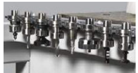
Tool changer 8- or 10 position tool changer on the side of machine chassis
