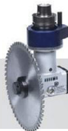
HSK F63 single angle cutter head, accepts a saw blade with one output, (ATLOCK-lock) max. Ø 240 mm Order no. 300-24-009 max. Ø 300 mm Order no. 300-24-008
