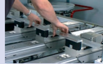
Special clamping elements for aluminium processing
