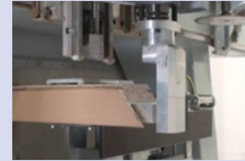
Drilling operation in a minimum of space for mitre joints used in door frames and architraves.
