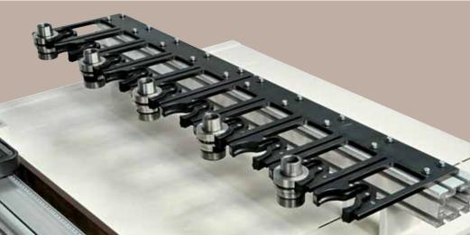
More flexible with fast couplings which can also be retrofitted, both for vertical and horizontal spindles.
