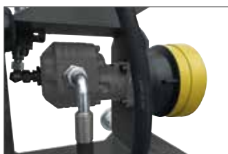
The ram stroke of all PTO models USP 13/16/22 is hydraulically controlled by an over-dimensioned cast-iron pump.
