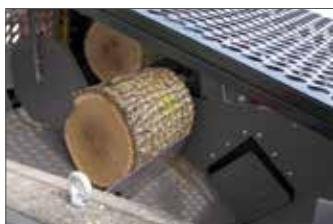
An hydraulic slider secures the logs and stops them from rolling down. Even if the last timber piece is too short, it will still roll down straight and centrally in the splitter carriage
