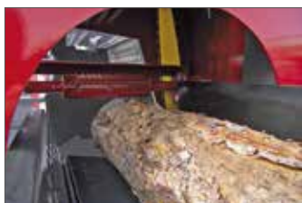
A push-down roll holds and secures the log in position while cutting is performed. This allows safe cutting of any timber to the very last piece.
