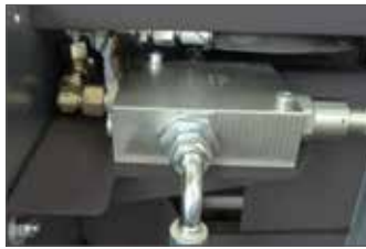
SSM 270 EZ: Differential valve for increased ram forward speed (fast splitting cycle).
