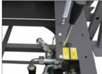
An hydraulic control valve is provided within operator's quick reach in order to switch the cutting blade on and off as needed.
