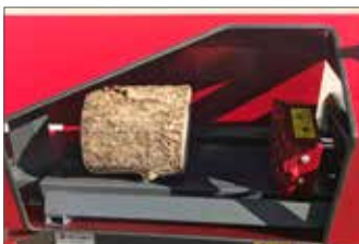
A manual adjustment screw allows safe stroke adjustment, and splitting of short logs at any intermediate position.
