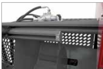
A hydraulic valve is available to allow stopping the infeed belt in the Stop-position. To set the log length (adjustable from 200 up to 600 mm / 7.9-23.6 in), simple move the valve by the required distance before starting to work.
