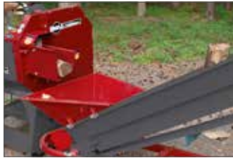
No more tilting of the carriage to the blade is needed. So, the log that is cut off the saw drops straight down into the hopper of the downstream belt conveyor.
