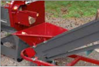
No more tilting of the carriage to the blade. So, the log that is cut off the saw drops straight down into the hopper of the downstream belt conveyor.
