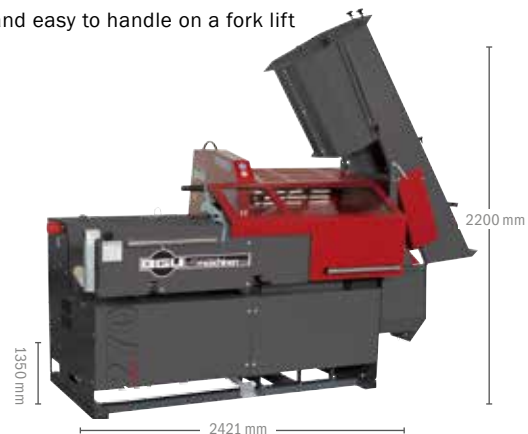
Transport asset with outlet spout folded up and timber infeed rollers retracted.
