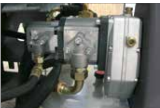
The fast forward speed of the hydraulic ram is made possible by the oversized hydraulic pump group III. A tandem pump is flanged to the main pump to power all ancillary functions as wedge lift and log lift operations.
