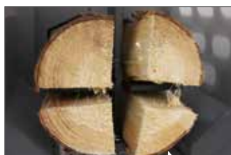
4-ways wedge: For a clean production of split logs, all in the same size.
