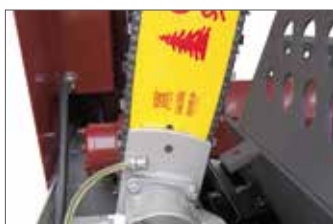
The saw chain is only engaged, after the descent of the chainsaw. So, no waste of oil and no early wear of the chainsaw bar will occur.
