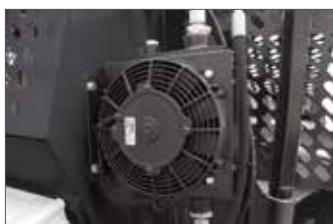
All KSA processors 455 EZ are equipped with a standard oil cooler.
