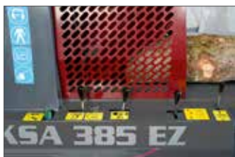
Ergonomic, easy accessible control board The descent speed of the chainsaw to and through the timber can be conveniently adjusted by means of a regulator (valve) installed on the control panel.
