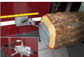
A hydraulic valve is available to stop the infeed table as needed. Before starting the machine, the valve settings can be changed to command cutting logs of the required length.
