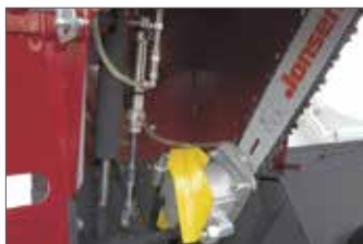
The saw chain is only engaged, after the descent of the chainsaw. This safety system has been designed for a longer life of the saw bar and chain at the same time.
