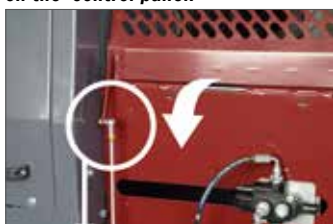
A safety valve stops all hydraulic functions and prevents accidental restart while the safety guard is lifted up. This additional safety ensures compliance to the EC norms and directives.
