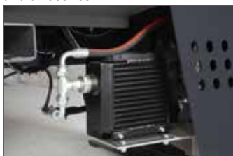
All processors model KSA 385 come with standard oil cooler to allow non-stop operation.
