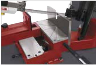
Mitre cuts are accurately adjustable at 90°, 45° and 60°.
