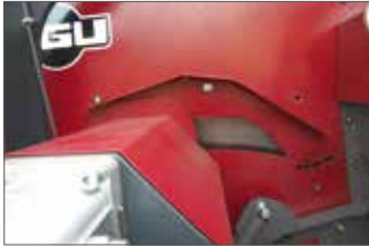
A special flexible guard on the saw arbor ensures top safety in all cutting positions. The blade teeth are always covered.
