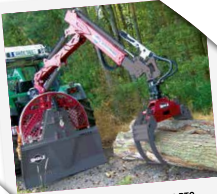
Timber loader with attached PTO logging winch.
