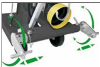
The lower linkage pins are adjustable in 8 positions by simply sliding them out or tipping them up/down as shown in the picture. This system provides for universal hitching to any kind of tractor.
