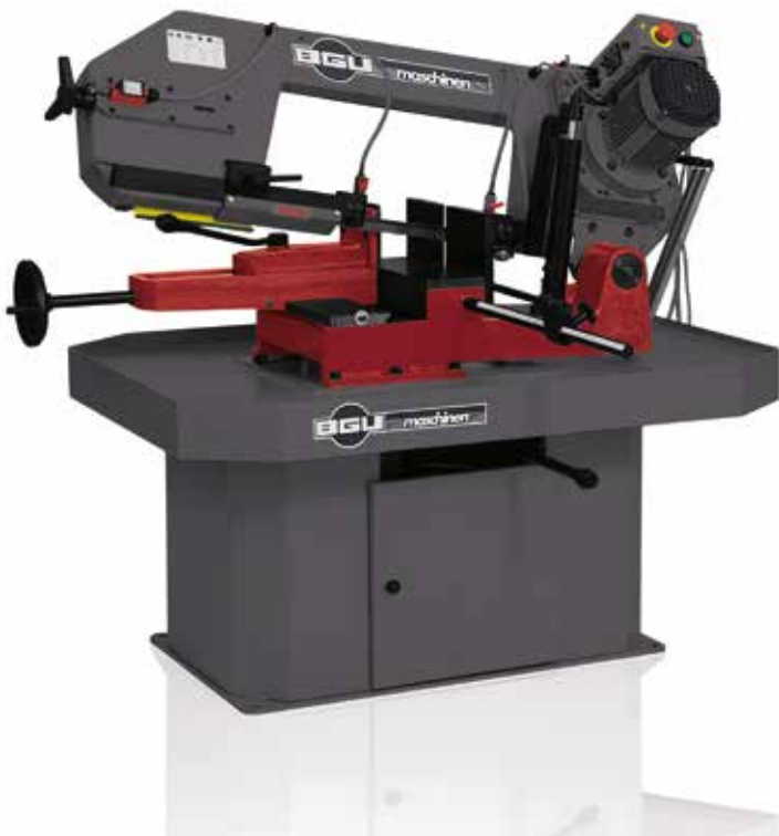
Mitre cuts are accurately adjustable at 90°, 45° and 60°.
