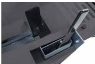
The splitter wedge can be quickly and safely raised/lowered to the required level by means of a control hand-lever.
