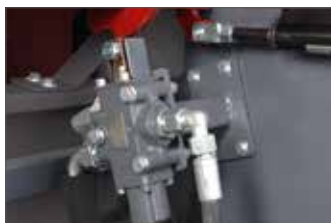
A safety valve prevents accidental restart of the splitter, while the safety guard is up-lifted.
