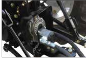
Model 700 Z with shaft-mounted gear pump (built-in hydraulics).
