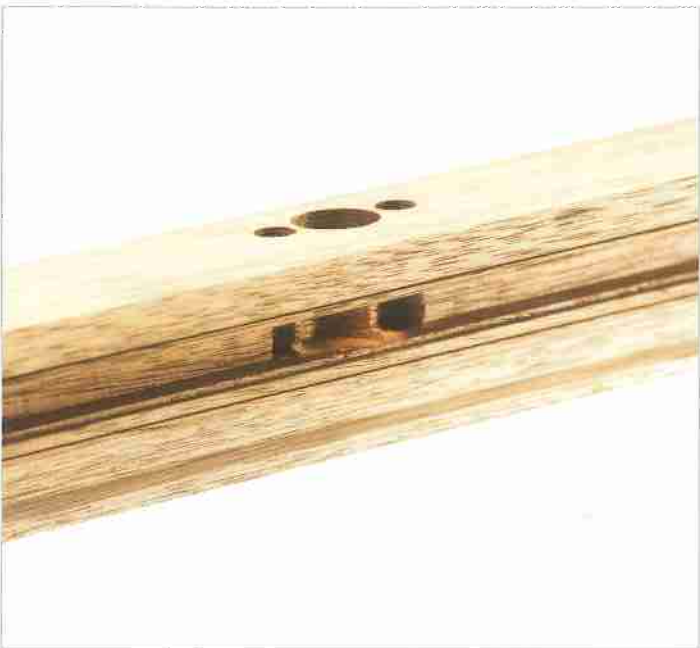
Complete machining of slots for hardware and fittings with no piece re-positioning.
