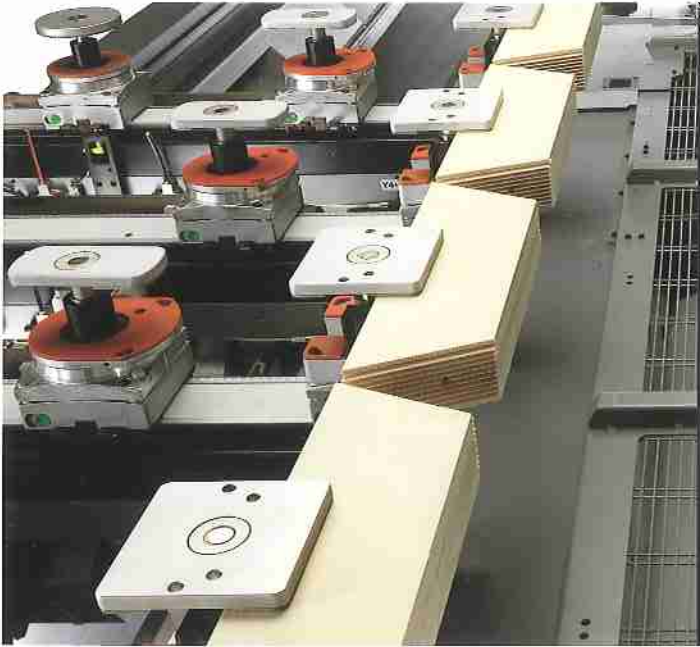
Working of arch segments starting from a single piece.
