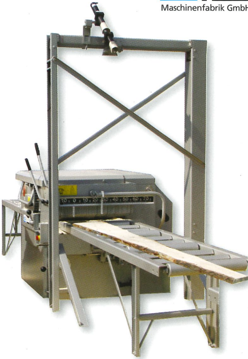
Series KME 2 edger with laser guide light
