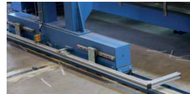
Run-over protection eliminates risk for personal injury when the nailing bridge is moving.
