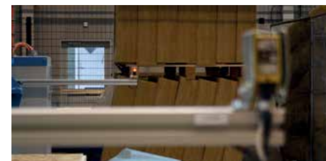
Light beams ensures that only the wall element is transported into the machine.
