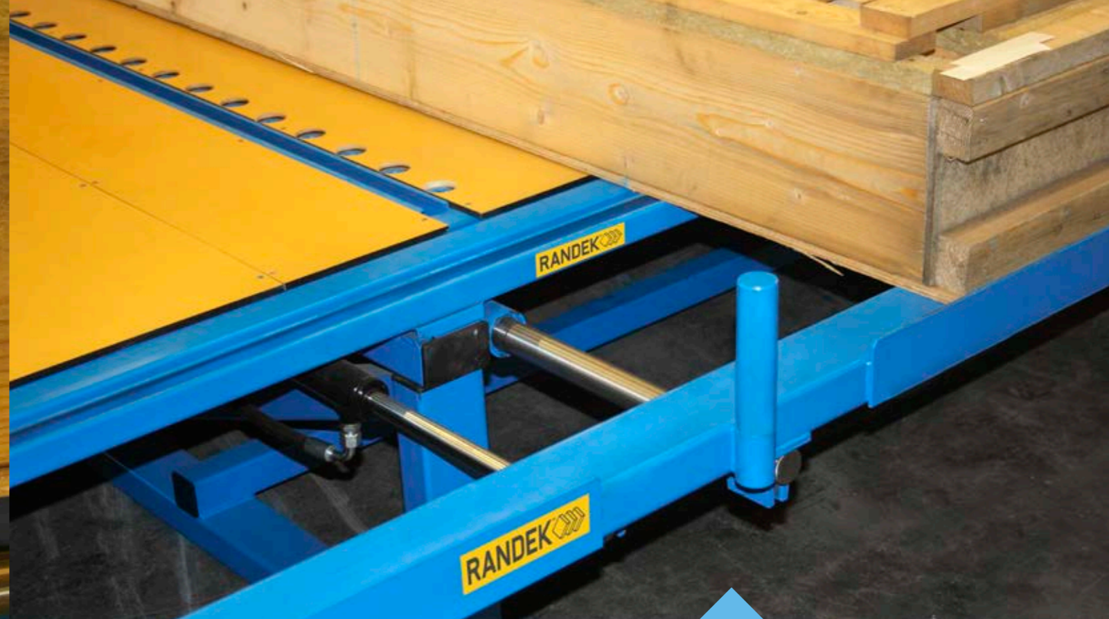
View showing hydraulic width and squaring function
