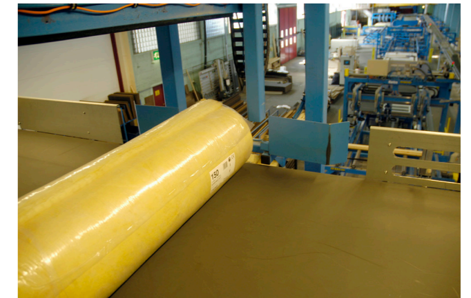
The insulation system can also be configured for handling of round packages of insulation.
