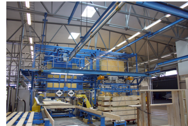
View over framing station FM3000 equipped with the world's most advanced system for handling of insulation.
