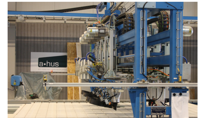
The nailing bridge is equipped with 8 nail pushers reaching a high capacity and batten straightener for positioning of the cladding.
