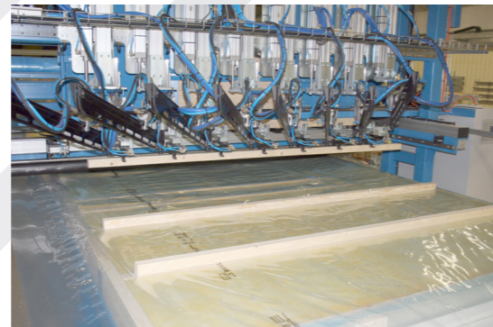
Placing and nailing of extra framework
