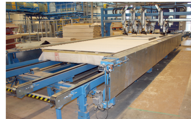
Nailing Table NTC3000 equipped with cladding template adjustable in x-, y-, and z-direction. The templates can easily be replaced.
