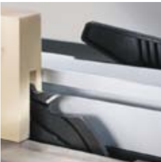
ts 4010 ci – operating with the adjustable groove cutter (SUVA guard is recommended for all hidden cuts)
