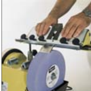
Jig 380 , to be used variably for knives with different width, precise, easy running and maintenance-free guiding by sliding bearings, hard anodized, fine-setting for grinding angles, 400 mm max. grinding length, Order no. 8949 0724
