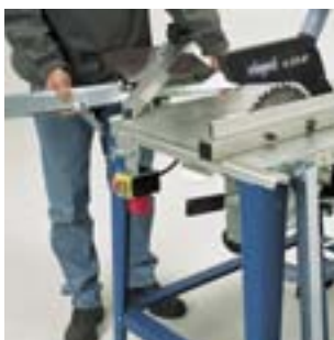
Optional patented "foldaway" panel cutting extension and removable sliding table carriage minimise workshop space. Ideal for transporting.
