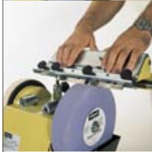
Jig 320 , for use with varying knife widths, especially for jointer and planer blades up to 320 mm, accurate, easy-running and maintenance-free sliding bearing guidance, hard-anodized, grinding angle fine-adjustment Order no. 8949 0723
