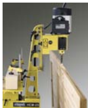
Door lock and hinge mortise holes are done by simply reversing the headstock position.
