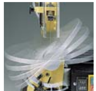
The saw table can be adjusted from 0 to 45 degrees.
