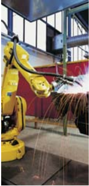
Metal fabrication is completed by a robotic welder. The robot's particular talent is repeated precision. When instructed correctly it never makes an error.
