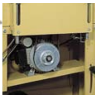
A powerful drive system enables the planing machine and optional attachments of operate separately.
