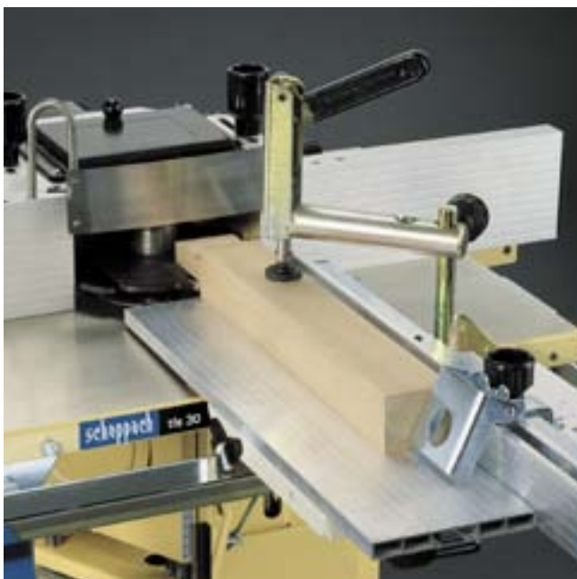
The tfe 30 spindle moulder attachment with sliding table carriage inclusive of tenoning table and clamp.
