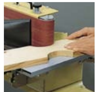
The small diameter of the end roller allows for perfect sanding of inner curves.
