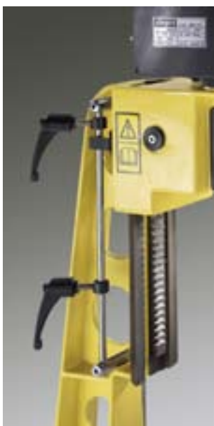
Mortise depth settings done through quick adjustment of easy lock levers.
