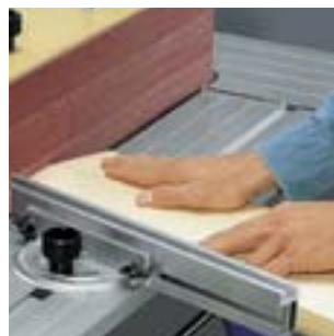
The angle fence can be adjusted to 45 degrees in left and right directions.
