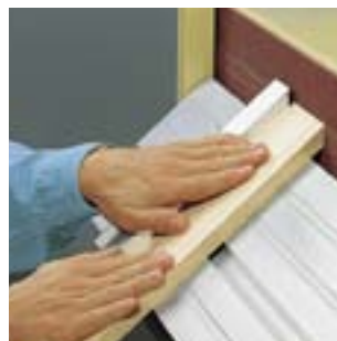
The angle fence can be adjusted to 45 degrees in left and right directions.
