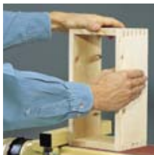
Assembled pieces can be comfortably sanded in the horizontal sanding mode.
