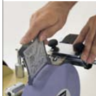
The angle guide 200/250 is used for measuring exact angles and settings 200: Order no. 8949 0717 250: Order no. 8949 0704
