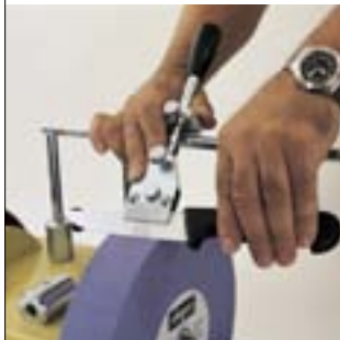
Jig 60 is suitable for small knives with blade length of 40 mm to 100 mm Order no. 8949 0708
