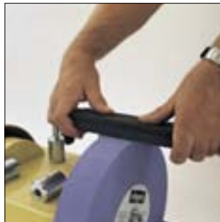
Stone grader changes the grains on the grinding wheel for fine abrasion Order no. 8949 0707
