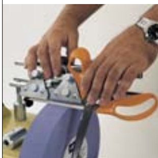
Jig 160 is designed for scissors and hedge shears Order no. 8949 0710
