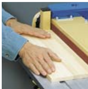
Assembled pieces can be comfortably sanded in the horizontal sanding mode.
