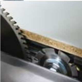
Scoring attachment (optional) for splinter free cutting of laminated and surface coated boards, MDF.
