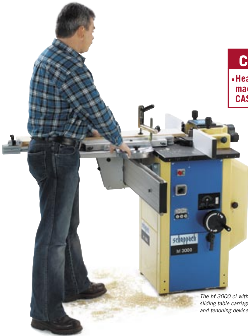
The optional tenoning cutting device allows you to work within 1/10th mm accuracy.
