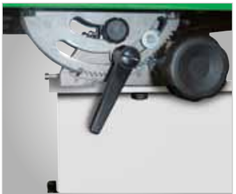
It is possible to incline the saw table on a rocker seat from 0° to 45°
