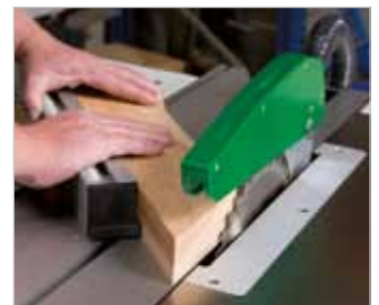
The cutting stop allows mitre cuts of 45° on both sides
