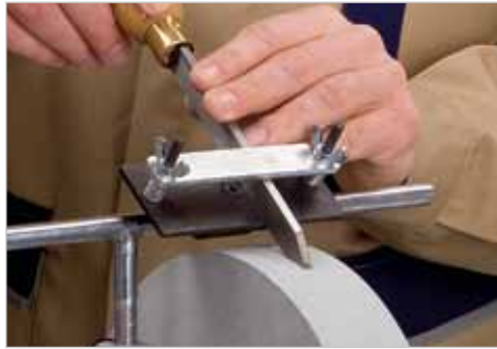
Sanding of cutting tools (Item No 591 0018)
