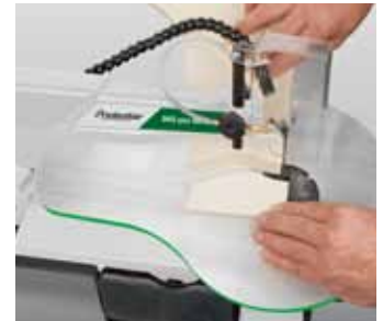
The large planed cast table can be inclined from -45° to +15°. The inclination is readable on a scale.
