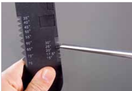
Step 1: Controlling and determining the cutting edge angle.
