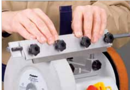
Sanding of cutting irons (Item No. 591 0024)
