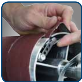
• Easy covering of the rollers without tools
