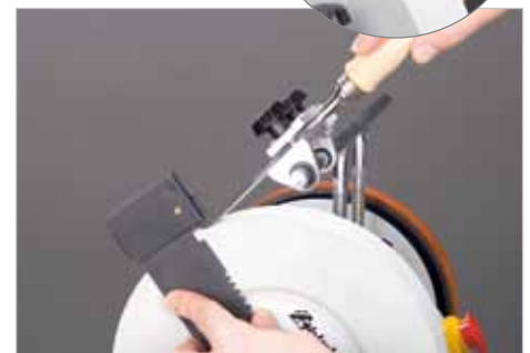
Step 3: Setting the appropriate clamp height for the cutting edge angle.
