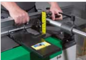
The aluminium planing stop can be infinitely inclined from 0° to 45°. The preset inclination is conveniently readable on a large scale.
