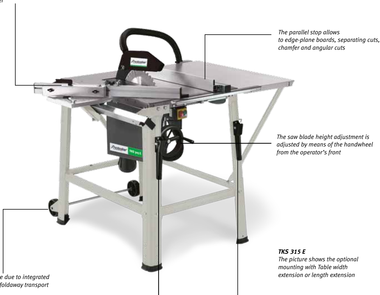
Ball bearing mounted sliding carriage with mitre stop infinitely adjustable from -45° to +45° with quick clamping lever
