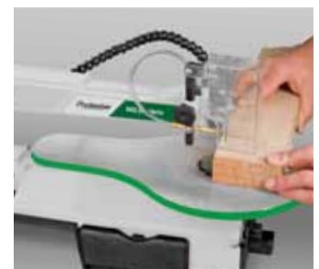
Work on wood pieces with a cutting height of up to 50 mm.
