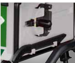
Mitre fence and bar pusher with handy brackets
