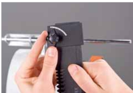
Step 2: Setting the measured cutting edge angle.
