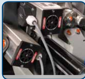
High frequency motors 13'200 min -1
