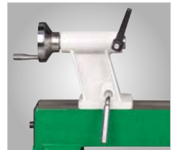
The tailstock made of grey cast iron is rapidly and easily fixed with a clamping lever. The adjustment of the centre sleeve is performed with a handwheel.
