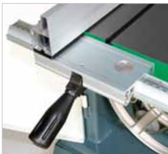
The aluminium parallel stop with eccentric quick clamping can be shifted easily and precisely. The preset value can be read off easily by means of an integrated magnifying lens together with a millimetre scale.
