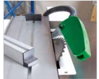
The saw blade is slewable by 45°.
