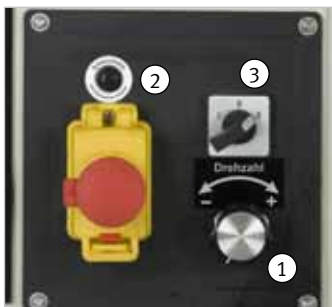
Variable speed regulation from 0-1'200 min -1 (L) and 0-3'200 min -1 (H) at two speed stages.
