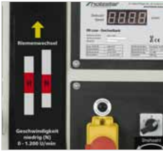
Variable speed regulation from 0-1'200 min -1 (L) and 0-3'200 min -1 (H) at two speed stages.
