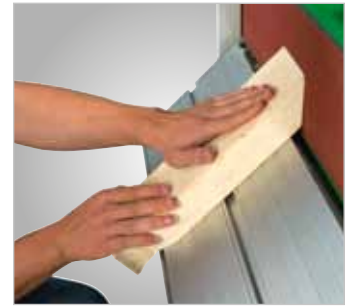
Mitres up to 45° by slewing the longitudinal table
