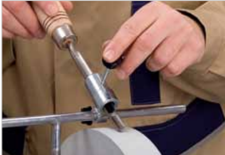
Sanding of gouges (Item No. 591 0021)
