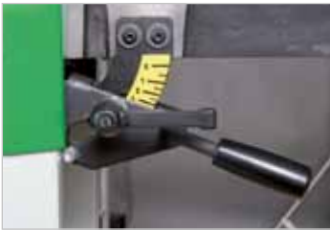
The height adjustment for the chip removal when planing can be easily set by a quick clamp (3 mm)
