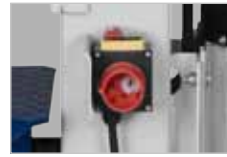
Switch/plug combination 400V/10A with phase inverter and overload protection as factory standard. (Fig. HSE 12)
