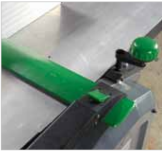
The plane iron is covered by a protection with handy quick clamping. The required chip removal for the thickener can be easily adjusted up to 2 mm on a handwheel. It is easily readable on a scale (Fig. shows ADH 250).
