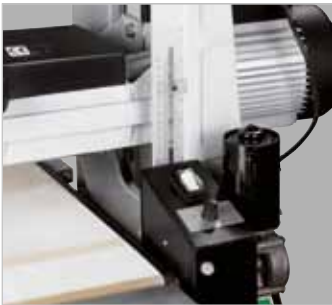
Height adjustment of the sanding unit readable on a scale
