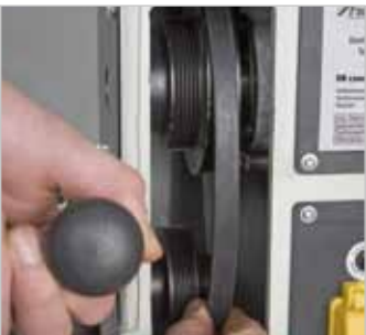
Changing the transmission stage by easy remounting the V-belt without tools
