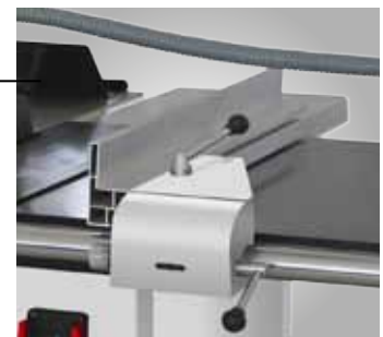
Large aluminium parallel stop on the round rod guide
