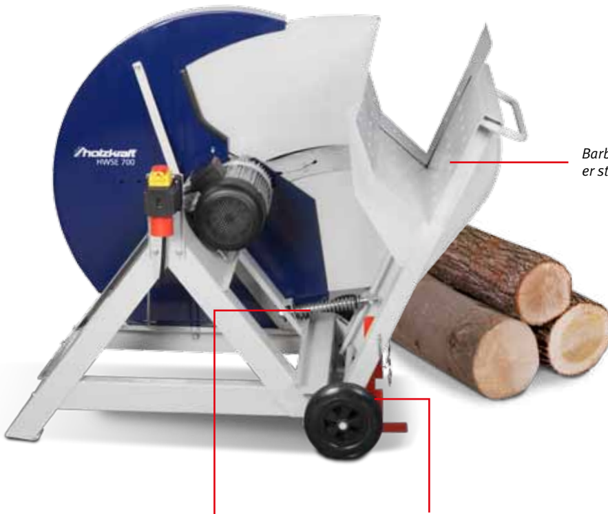
Automatic rocker return unit via spring balancers
