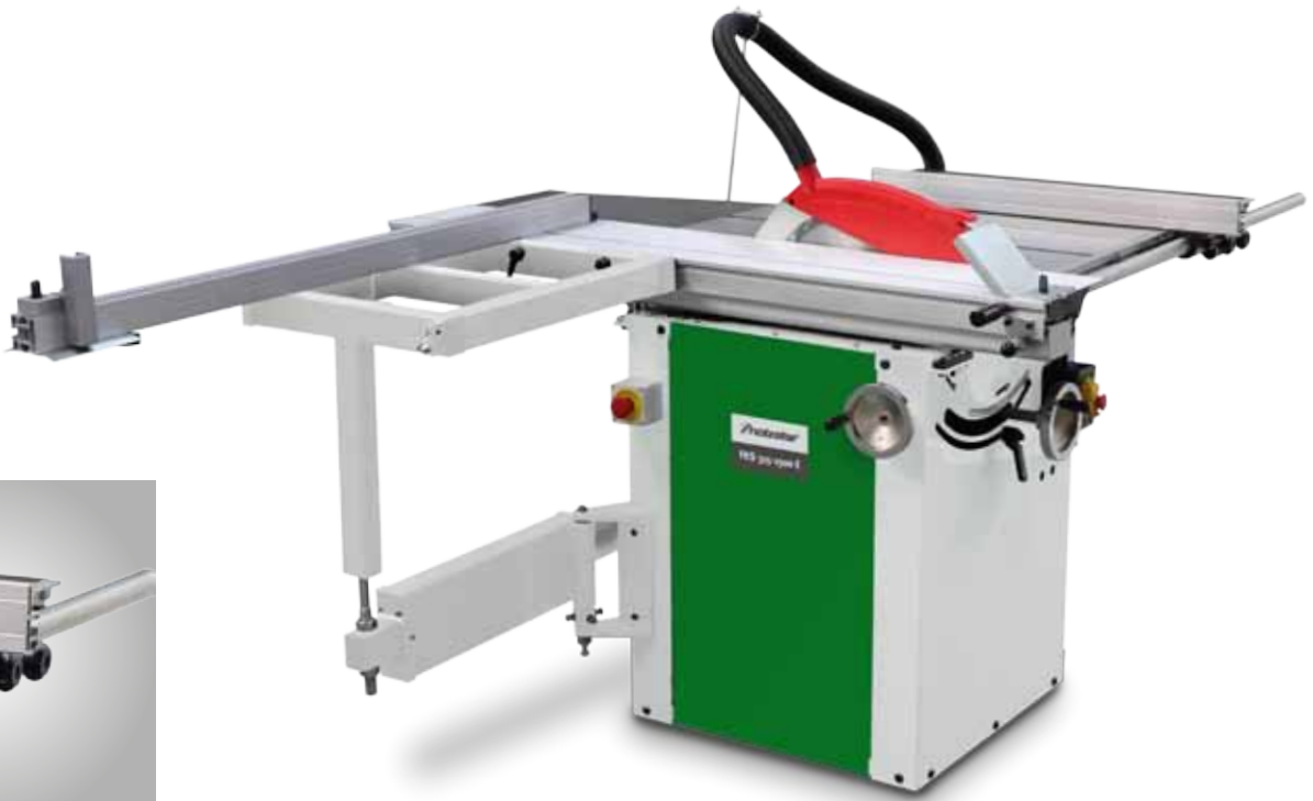
Large aluminium parallel stop on the round rod guide including eccentric quick-clamping
