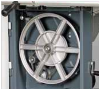
The 2-level speed adjustment is performed manually by simple displacing the belt on the HBS 351-2. Equipped with chip brush for neat running surfaces of the driving wheels.
