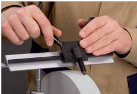
Trimming the grindstone (Item No. 591 0029)
