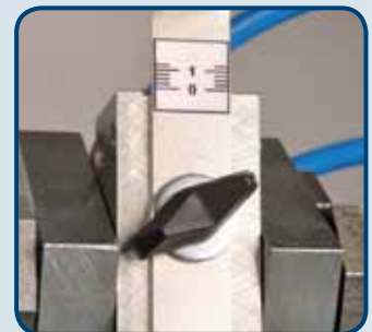
Chopping unit with fine adjustment of the cutting length
