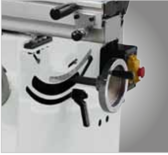
Saw blade slewing from 0° to 45°, conveniently adjustable by means of a rotary knob and a scale with toothed rack mechanism
