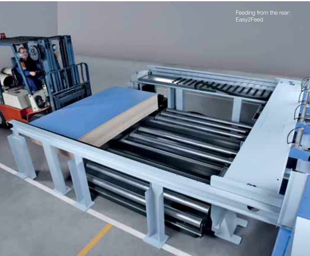
Feeding from the rear: two-tier roller conveyor
