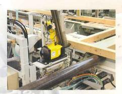
the NC-controlled discharge gripper which moves exactly to the single stud positions. Another innovation are the freely definable nailing positions for different stud types such as L, U, T or multiple studs.
