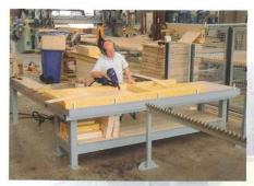
The module production line consists of a module table, a module transport way and a module support.
