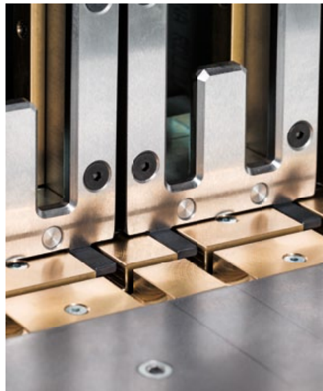
Interchangeable cutting lips made of non-ferrous metal.
