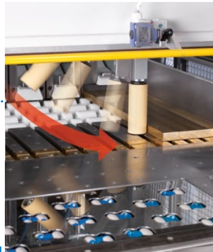
Pneumatically controlled vertical fastening unit for strip cuts.
