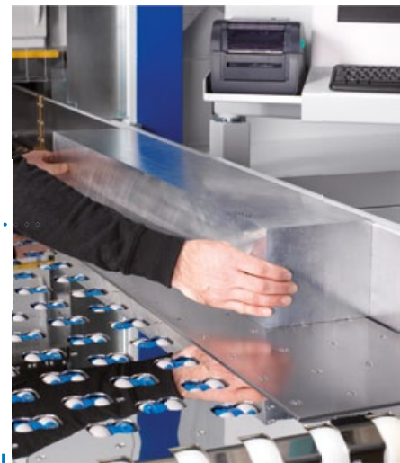
Angular table with air cushions and rollers on all sides for energy-saving material handling.
