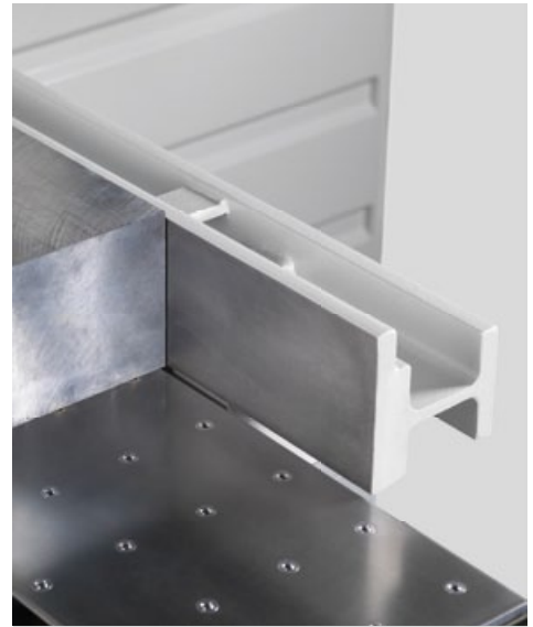
Ergonomic air cushion table with a long angle stop for easy operation and high angular accuracy at the cutting line.
