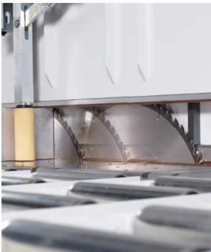
Split pressure beam for perfect extraction results when cutting.
