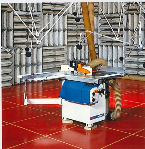
CSR (Reserch and development dept. SCM GROUP) – Semi-anechoic room.
