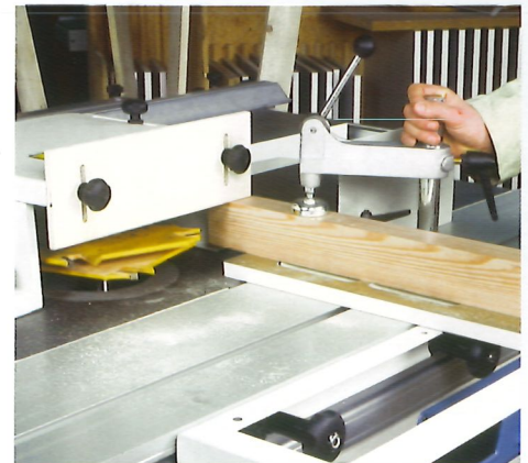
Tenoning unit consisting of a tenoning table, guard for tools with diameter up to 275 mm and an extractor hood (diameter 120 mm)
