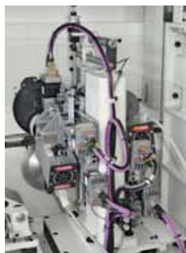
RSU -HD Minimum interaction with the panel due to movements on linear guides with recirculating balls. xd
