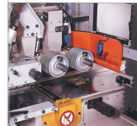
UPPER AND LOWER INFEED WITH PNEUMATIC CONTROL Rollers are powered, providing pneumatic control and a pressure gauge for a smooth feeding effect. A limit switch prevents feeding from oversized stock.
