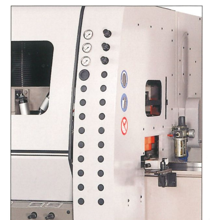
INDIVIDUAL ADJUSTABLE PNEUMATIC PRESSURE GAUGES FOR POWERED FEEDING ROLLERS
