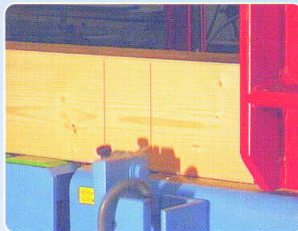
Rafter markings can be made on all 4 part sides
