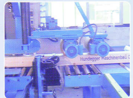
On-the-fly inkjet marking system - marking and labeling possible on three part sides.
