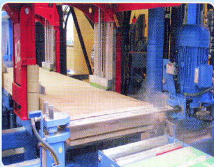
The guided slot cutter can accurately make through-slots of any length on parts up to 625 mm wide as well as blind slots from the fence side.
