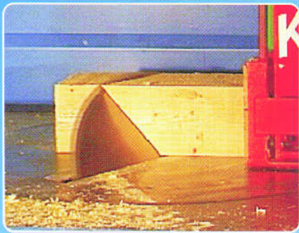
Various types of jack rafter cuts
