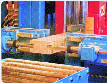
Splinter-free drilling and milling is made possible with the double support feature. Processing both sides simultaneously, without having to rotate the timber, greatly reduces cycle time.
