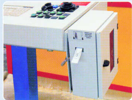
Console printer creates labels with part name, part number, etc.
