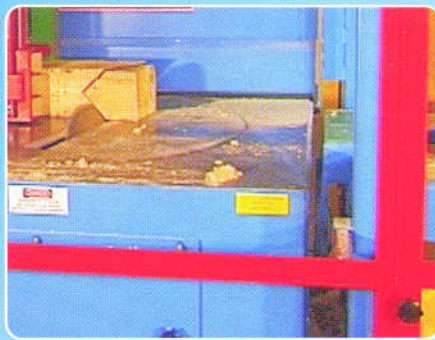
V-cuts of any angle and depth
