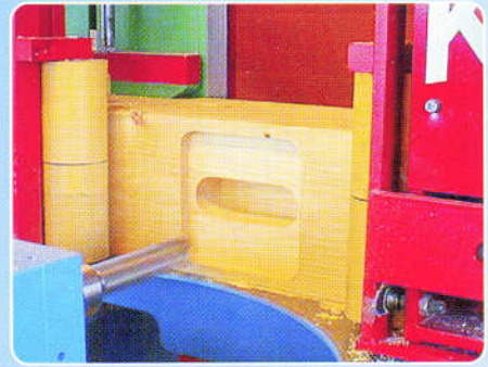
Housed tenon connections
