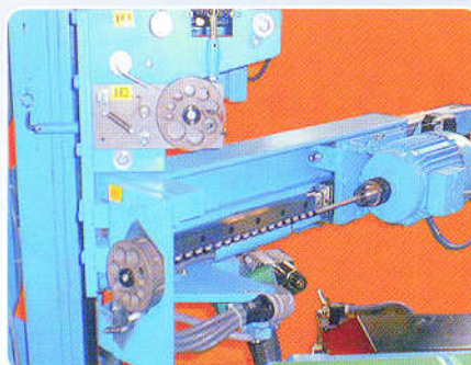
Angled horizontal drill unit.
