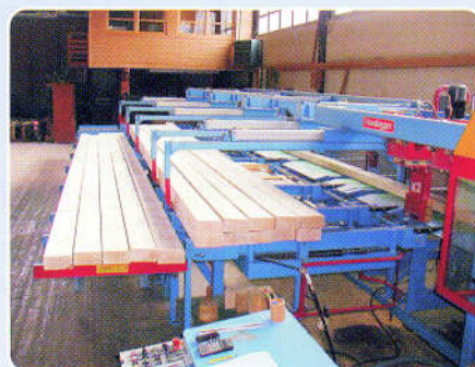
Hydraulic lift table with automatic de-stacking unit
