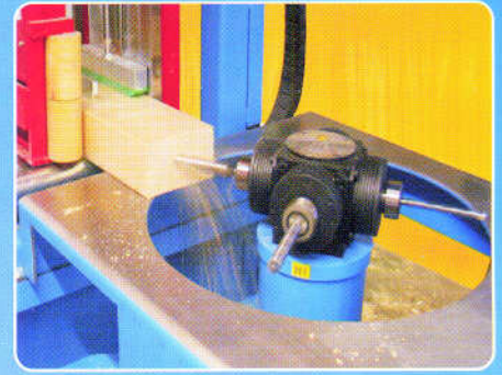
Revolving Mill - Horizontal. Capable of using up to 4 different tools, like drills, end mills, rolling cutters or dove tail cutters.
