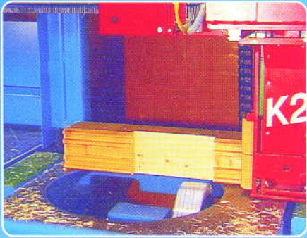
Seat cuts at any angle on all four part sides
