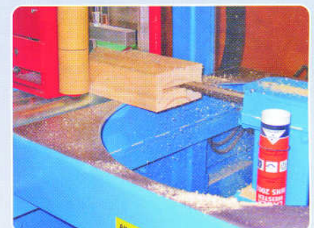
Blind and angled slots can be easily produced with new beam end slot cutter - 360° angled.
