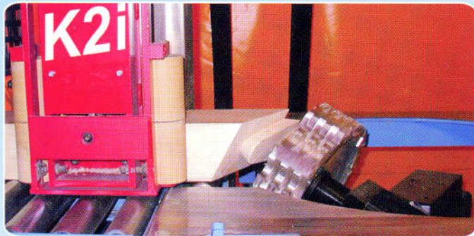
Dovetail connections on jack rafters can be accurately processed at any angle or bevel using the 5-axis mill.
