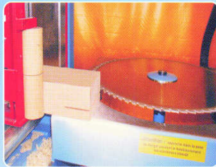
Dados up to 300 mm deep can be quickly and cleanly produced with the horizontal saw.
