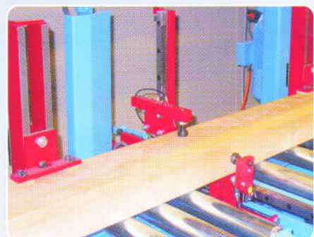
Dimensional measuring for auto recognition and correction of rough timber dimensions
