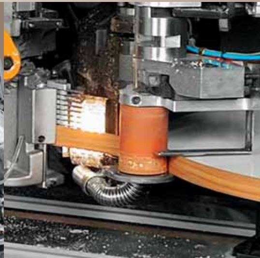
High performance edgebanding unit for glue applying straightly on the panel.
