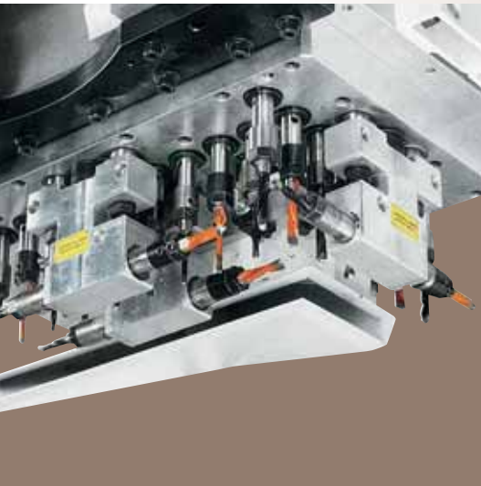
Boring units with 18 vertical and 6 horizontal spindles.
