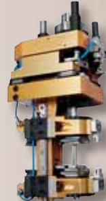
Multifunction trimming unit for thin edges + gluescraping
