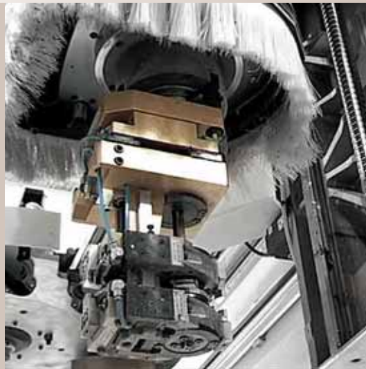
4 or 5 axes electrospindles of last generation with a power-rate of 13 kW (in S1 working cycle) to carry out all machining with the maximum precision and finishing quality. Great housing of tools thanks to 28 positions in tool-room.
