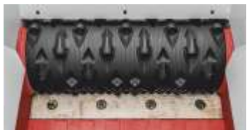
Rotor-Version 8 (30 mm Knife-Ø)
