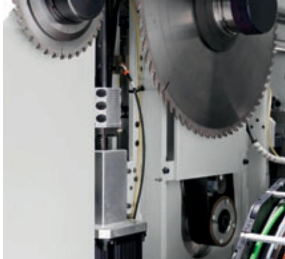
The blades raising is obtained by a Brushless motor and a ball screw system. This system guarantees both accuracy and rapidity in the blade projection adjustment.
