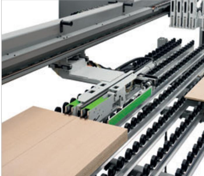
An auxiliary pusher composed by two independent grippers with numeric controlled side positioning. An additional side support permits to cross cut independently strip up to 1200 mm wide.
