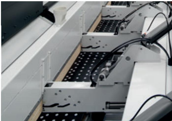
The pressure beam has a single structure for an even controlled pressure on the stack of panels to be cut. The closing of the grippers passages is guaranteed by a gravity system.
