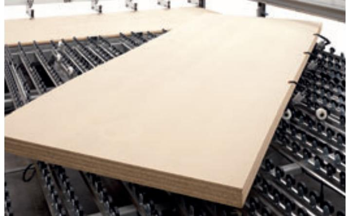
Turning station (Selco patent) for the rotation of the stack of panels keeping the alignment to the reference point before and after the rotation. Panel clamping devices avoid the misaligning of the stack during the rotation phase. The stack of panels is aligned before and after the rotation with two separate groups of squaring devices.
