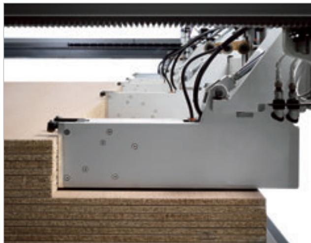
The independent self-levelling grippers assure the firm clamping of the stack of panels. Their special structure and the machine logic allow the total ejection of the stack of panel beyond the cutting line, thus facilitating their movement and the unloading of the trim cuts produced.
