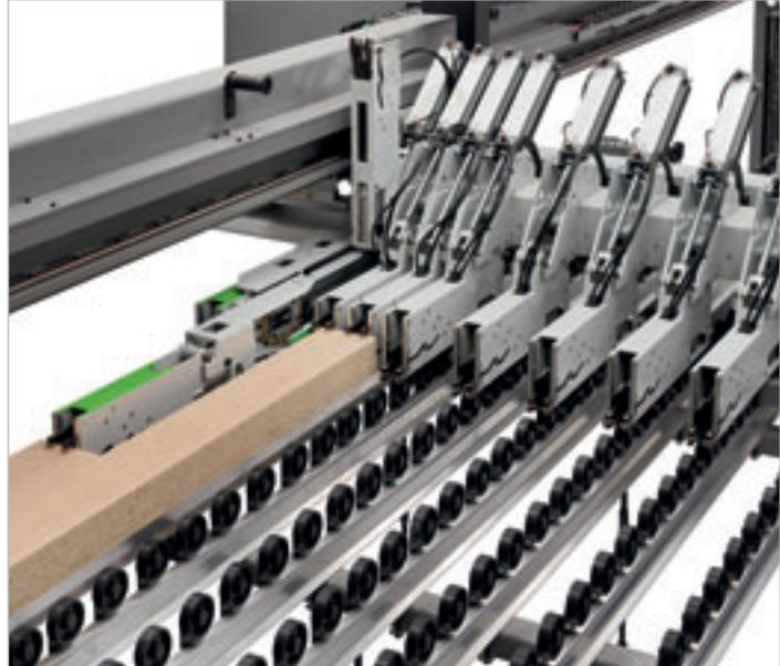
Staggered cross cutting of narrow strips.
