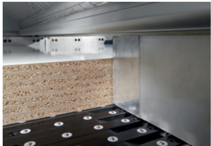
A new-concept side aligner (patented) located inside the pressure beam aligns the material, exerting a pressure in the point where the cut has to be made.
