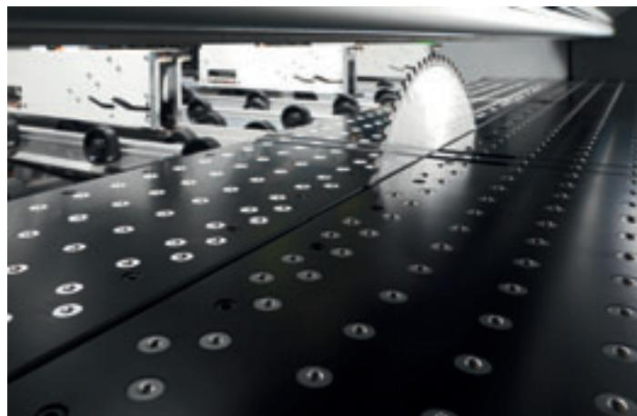
Main machine frame with air jet for gentle handling of delicate materials. It cleans as well the machine table around the blade.
