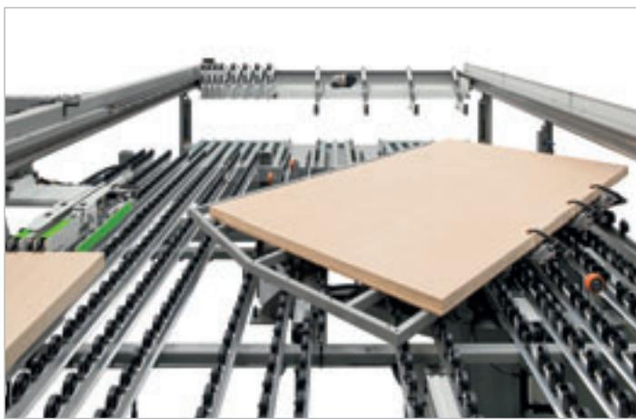
Cross cutting of the last strip while loading and rotating the next stack of panels to be cut.
