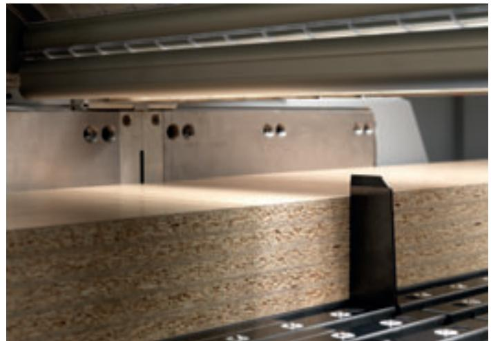
The side aligner is integrated with the saw carriage. Its characteristics align perfectly even thin or flexible panels reducing cycle cutting time.
