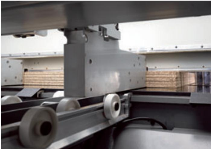
The pressure beam has a dual structure for an even controlled pressure on the stack of panels to be cut.
