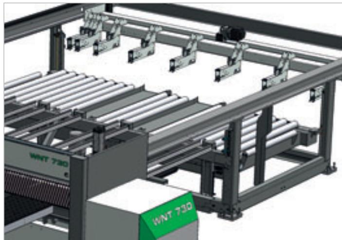
The heavy duty pusher carriage for precise and fast panel positioning is driven by a brushless motor. The supporting table under the pusher carriage is equipped with idle independent rollers to avoid any scratching on panels with delicate surfaces.
