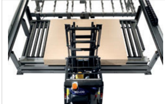
The lift table consists of a strong frame raised and kept perfectly levelled by four bronze volutes and steel screws simultaneously moved by a gear box. The frame is equipped with a special structure to load the pile of panels directly by forklift.
