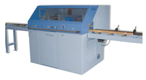
Loghouse milling machine Blockhausfräse BL100 for economic production of components used in modern log cabin construction.
