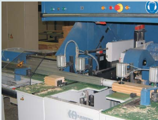
BL100A Servopusher zur Werkstückpositionierung BL100A Servopusher for workpiece positioning
