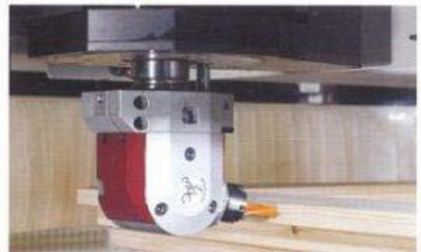
■ Inclined boring for door hinges.
