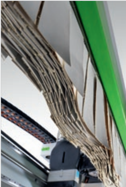
Side curtain guards to protect the working unit, which can be moved to enable the machine to work at maximum speed in total safety.
