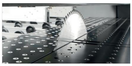
Top product quality, thanks to the air cushioned working surface, which protects delicate materials. In addition, this characteristic ensures the surface next to the blade is kept constantly clean.
