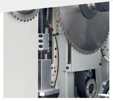
Vertical movement of the main blade is managed and optimized via quick blade height adjustment.
