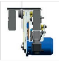
The excellent balancing of the tool-holder carriage (thanks to the shape of the base and the positioning of the guides and wheels) means there are no blade vibrations at all, and the carriage makes an extremely linear movement.
