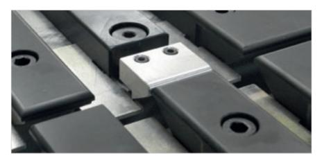
**Cutting line closure system**, to prevent the longitudinal trim cuts from falling into the machine and fouling the blade path.
