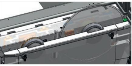
The **anti-slide device** controls the position and the number of rotations of the blade, intervening to adjust the advance speed. Maximum cutting quality, a longer blade lifespan, and reduced maintenance costs.
