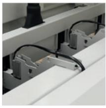
The consistent, controlled pressure on the book of panels to be cut is guaranteed by the **presser** with its single-element structure.
