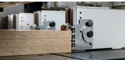
**Collets with specific stops** for processing books of laminated materials with protruding edges.
