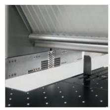
Perfect alignment of very thin and/or flexible panels too, minimising cycle times thanks to the **side alignment** stop integrated in the blade carriage.
