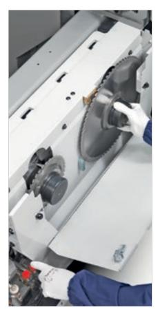
**Quick Change system** (patented) for the quick release of the blades without tools.
