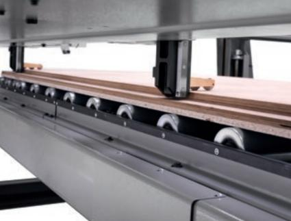
Thin panels can be loaded from the lifting table, using independent floating pushing points that are electronically controlled. A specific logic together with the front pop-up stops prevent the risk of mis-feeding (by means of attrition) those panels that don't belong to the book being fed.
