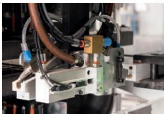
System of glue injection and dowel insertion with two opposing units, for machining the two ends of the panel.
