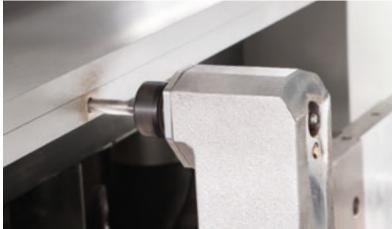
THE MACHINE CAN BE FITTED WITH ONE OR TWO INDEPENDENT HORIZONTAL UNITS.
