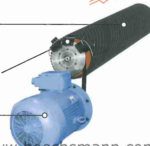
Pneumatic operated disk brakes to stop the working units within few seconds from emergency.
