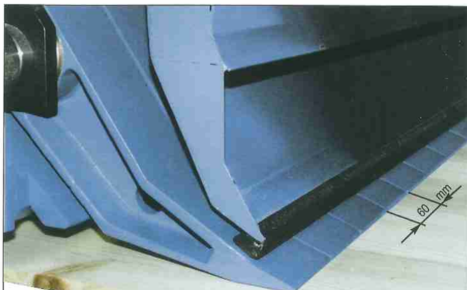
Infeed sectioned pressure unit + dust hood intake
