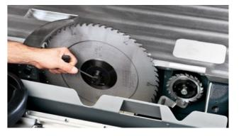
**Simple, safe & quick – "Quick-lock" saw blade clamping** Quick and easy blade change with only one tool, thanks to the "Quick-lock" system.
