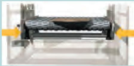
**Table lifting system:** Innovative conveyor table lifting system by means of four pistons and integrated with a further table retention system on the four specially worked and ground sides of the bed. This system provides a standard of strength and precision that is unique in the calibration-sanding machine industry.
