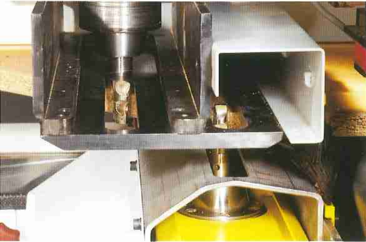
CF 10: With greater profile depths, the rough contour is created in line with the prescribed path using two finger cutters.
