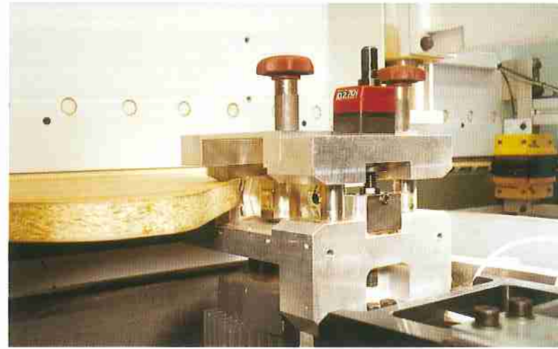
CF 12: Two units trim in synchronous and counter rotation to achieve a neat, tidy contour.
