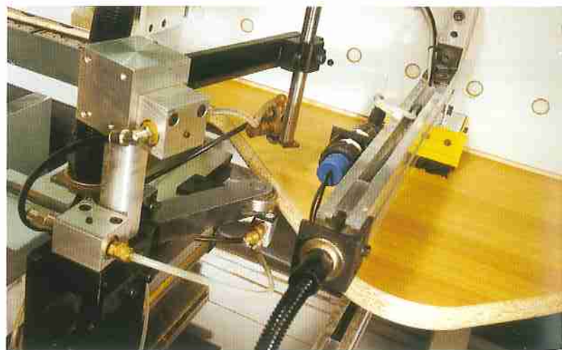
Separating agent is sprayed on to ensure optimum quality of the glued joint.
