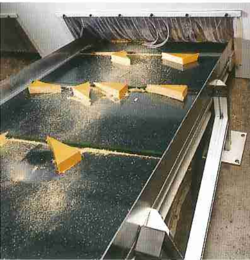
Separating agent is sprayed on to ensure optimum quality of the glued joint.
