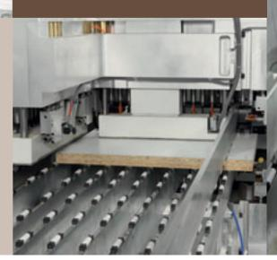
The new panel hold-down grippers feature a revised geometry and independent movement to also allow drilling operations in positions inside the gripper area, for an improved optimisation of the machining of the workpiece and a reduction in the cycle times.
