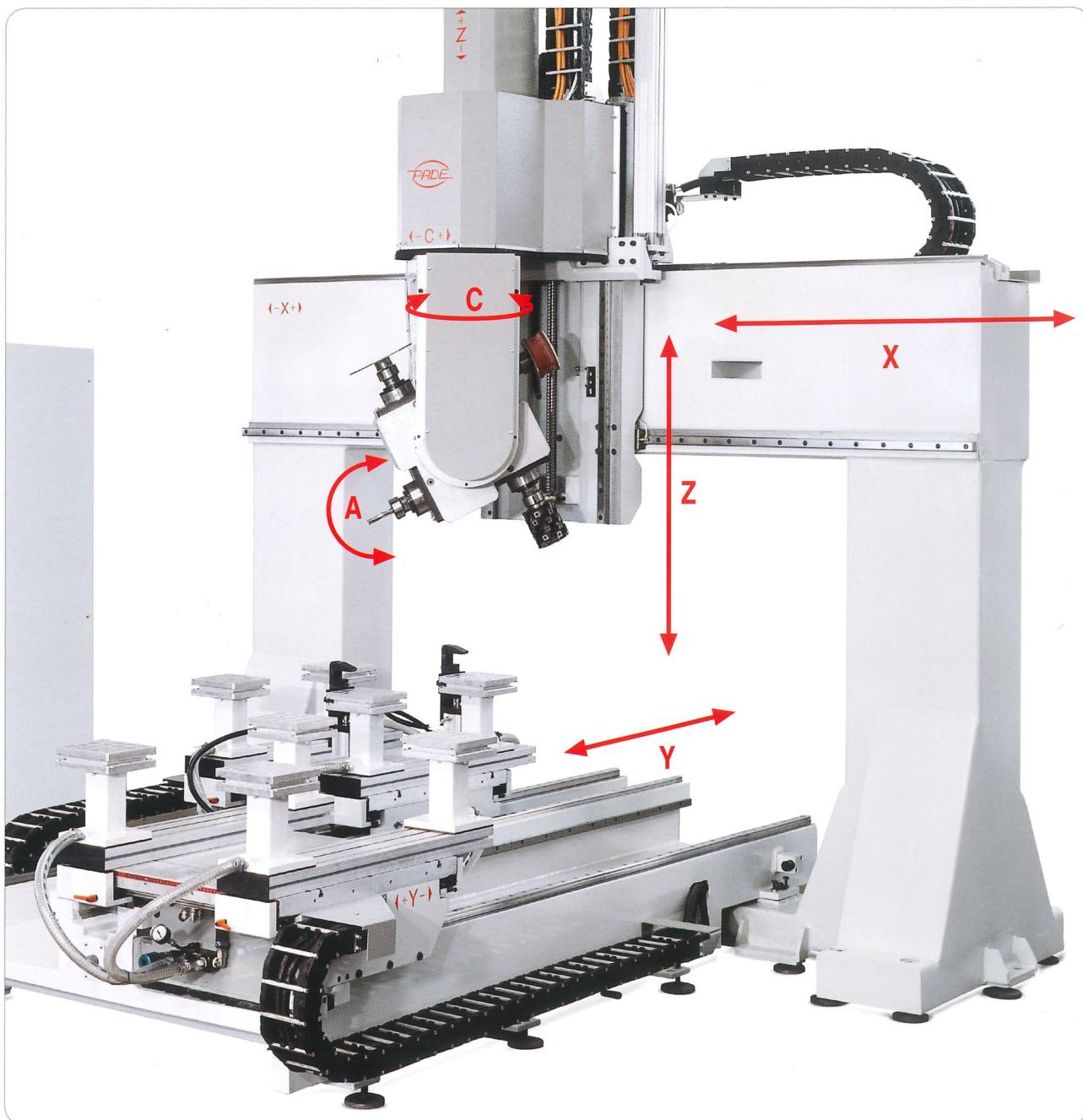
**CLIPPER** is the open beam structure workcenter particularly meeting the high standards of manufacturing chair and table components as well as solid wood elements in general. It has been designed for precise 5 axes interpolated machining operations: boring, mortising, tenoning, shaping with unrestricted three-dimensional manoeuverability. The dynamic conception of CLIPPER offers a higher degree of flexibility ideally suited to machining also plastic articles.
