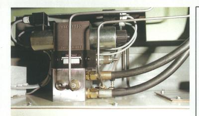
All **SAVI** guillotines are equipped with a central hydraulic block system, that minimizes the risk of leakages.
