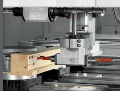
machining head: auxiliary unit for boring and routing
