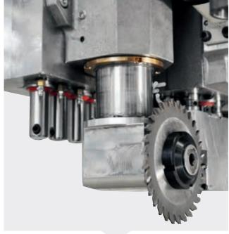
The optimum solution to all boring requirements is found in the wide range of modules available for the Accord fx, with from 14 to 50 independent spindles.
