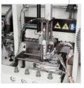
**ROUND 1 rounding** unit: rounding of corners on straight and shaped panels.
