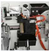
Perfect junction line and use of EVA and PUR glue thanks to the "SGP" glue tank.
