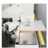
Easy size: infeed guide with axis for the NC adjustment of the material removing of the pre-milling unit.
