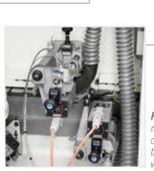
R-K trimming unit: rapid machining changeover between thin, thick and solid wood edges.
