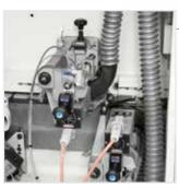
**R-K trimming unit:** rapid machining changeover between thin, thick and solid wood edges.
