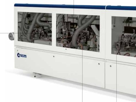
Pressure roller conveyor with electronic positioning and timed intervention.
