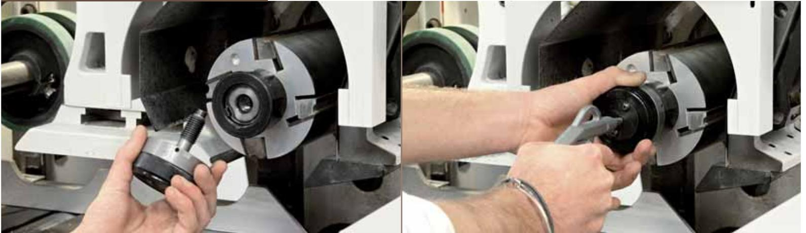
**T-SET: device for tool locking/unlocking**
