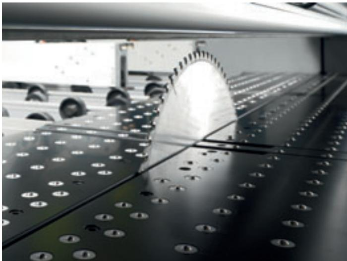
Main machine frame with air jet for gentle handling of delicate materials. It cleans as well the machine table around the blade.
