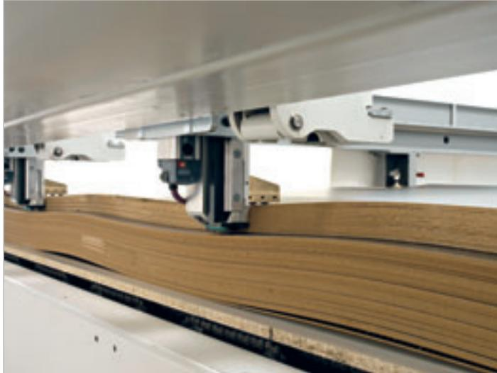
Thin and corrugated panels can be loaded from the lift table through the use of special electronic controlled oscillating pushing points. A specific taking over logic and stopping devices (patented) avoid that the thin material panels below the actually loaded stack are drawn by friction during the loading cycle.
