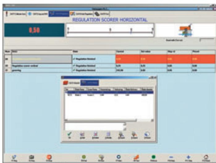
Electronic adjustment of scoring saw blade by means of the Digiset electronic device. This system is used to memorize and recall the aligning positions of saw blade sets, thus making extremely fast and precise the saw blades alignment after sharpening.
