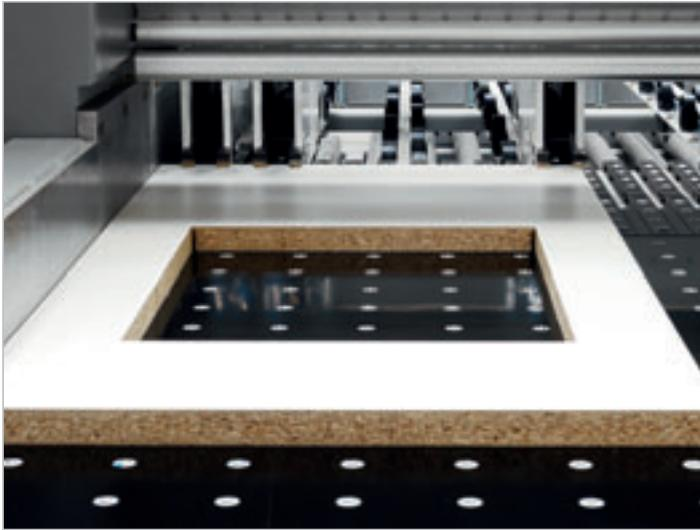
**Software for executing window openings on panels. The various patterns can be stored on the numeric control.**
