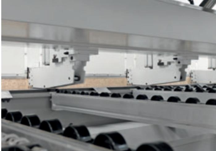
The pressure beam has a single structure for an even pressure on the stack of panels to be cut. The closing of the grippers passages is guaranteed by a gravity system.
