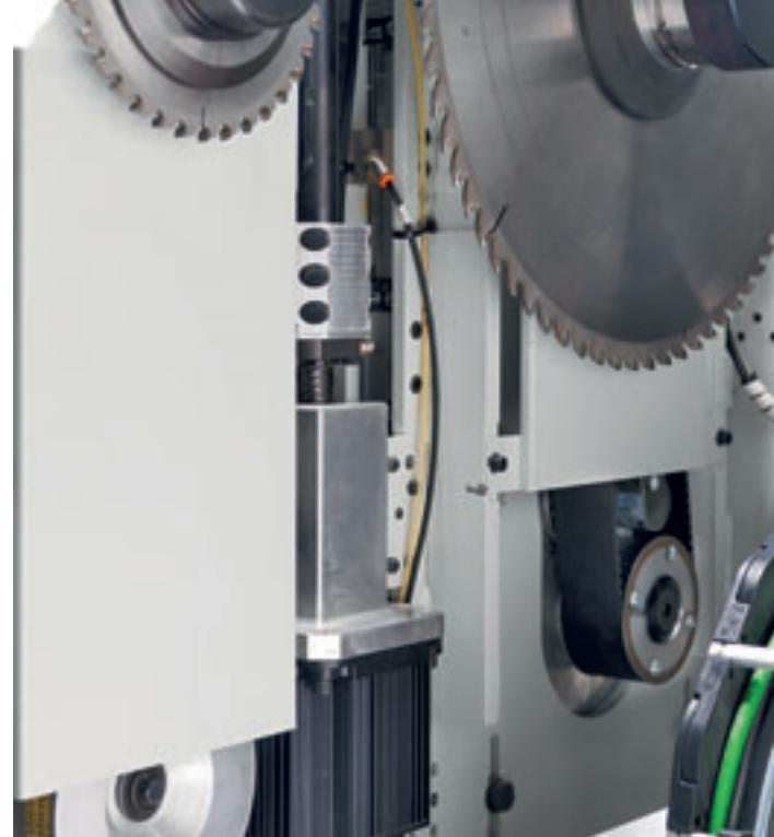
The blades raising is obtained by a Brushless motor and a ball screw system. This system guarantees both accuracy and rapidity in the blade projection adjustment.
