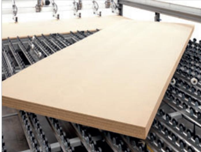
Turning station (Selco patent) for the rotation of the stack of panels keeping the alignment to the reference point before and after the rotation.
