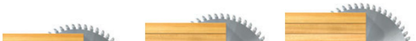
The main saw blade projection and the pressure beam stroke are automatically adjusted by the numerical control in relation to the thickness of the stack to be cut, thus obtaining the best cutting quality under any working condition.
