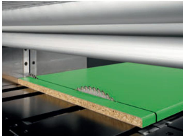
**Device for the automatic execution of grooves whose width may be programmed by the numeric control. The groove depth may be manually adjusted from outside the machine with saw blades in motion or by means of an electronic device.**
