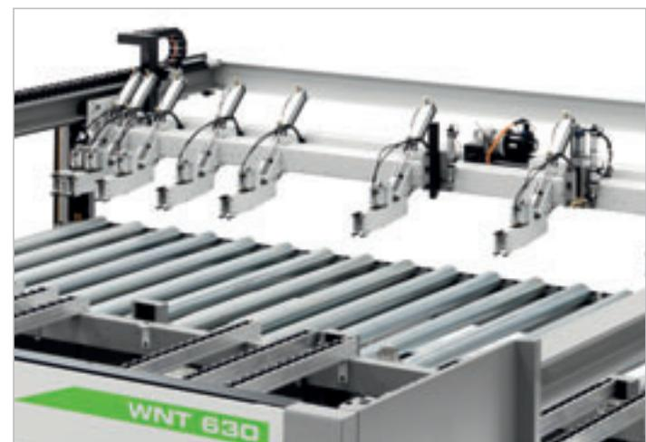
The independent self-levelling grippers assure the firm clamping of the stack of panels. Their special structure and the machine logic allow the total ejection of the stack of panel beyond the cutting line, thus facilitating their movement and the unloading of the trim cuts produced.
