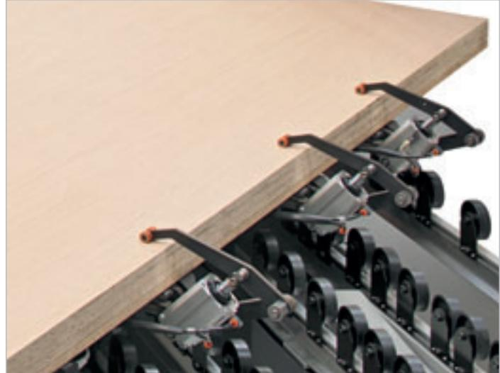
Panel clamping devices avoid the misaligning of the stack during the rotation phase (option).
