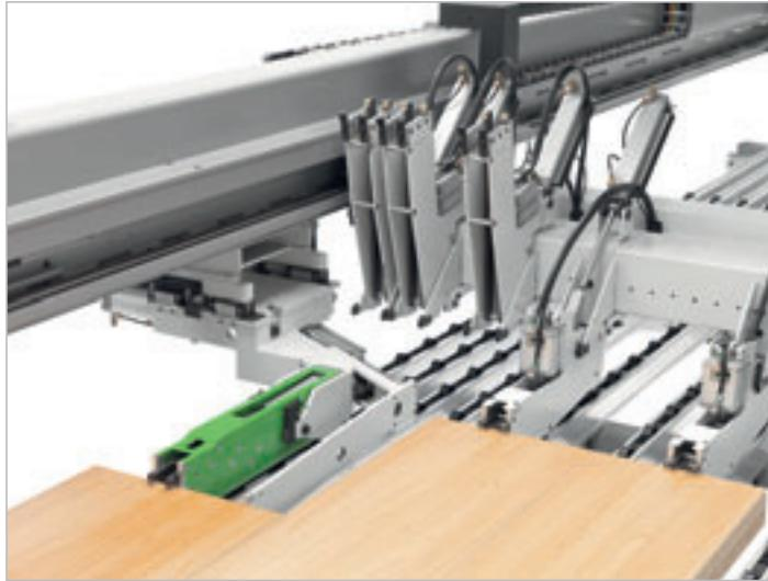
**Auxiliary pusher composed by one gripper with numeric controlled side positioning. An additional side support permits to cross cut independently strip up to 600 mm wide.**
