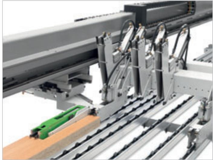
**Staggered cross cutting of narrow strips.**
