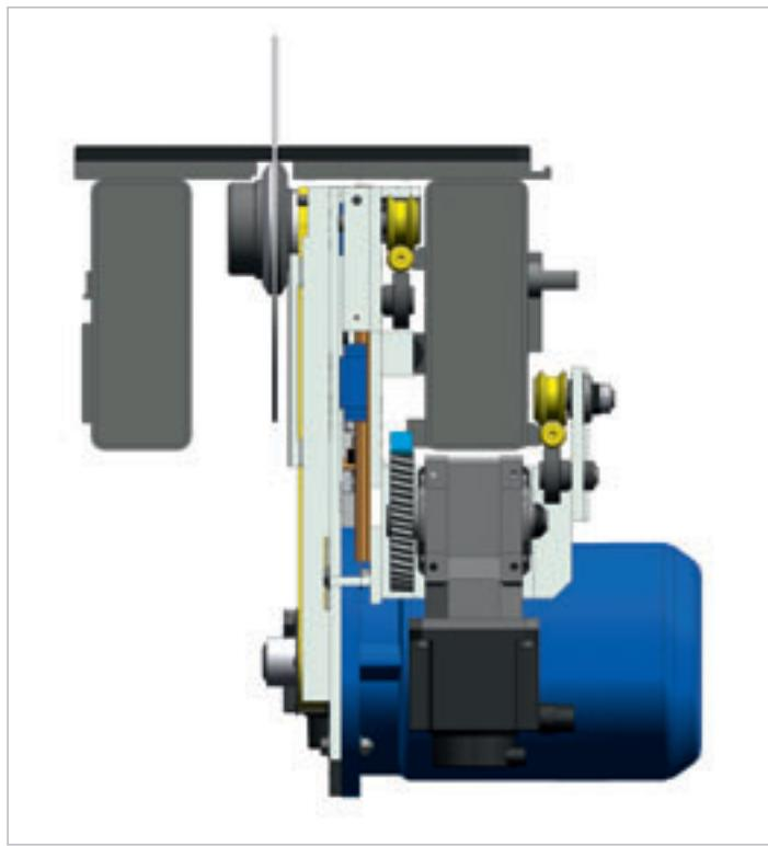
The special base structure and the positioning of the guideways and guide rollers assure an optimal weight balance of the saw carriage. The absence of saw blade vibrations is granted by the top guide which is positioned right beside the saw blade hub. The extremely linear movement of the saw carriage is obtained by a rack and pinion system and by a brushless motor installed on the saw carriage itself.
