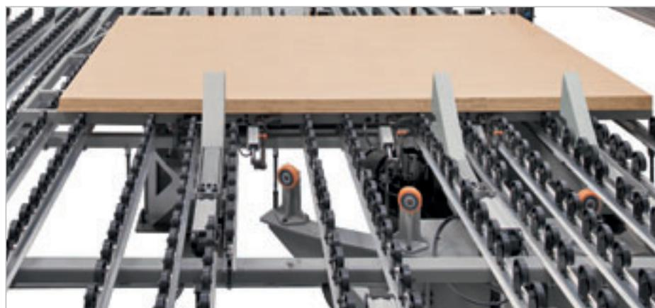
Front aligners to align the boards in the width directly on the turn station unit (option).
