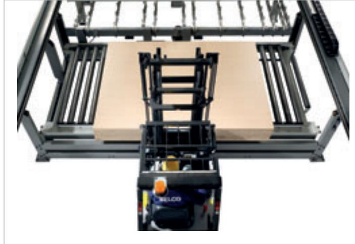
The lift table consists of a strong frame raised and kept perfectly levelled by four bronze volutes and steel screws simultaneously moved by a gear box. The frame is equipped with a special structure to load the pile of panels directly by forklift.
