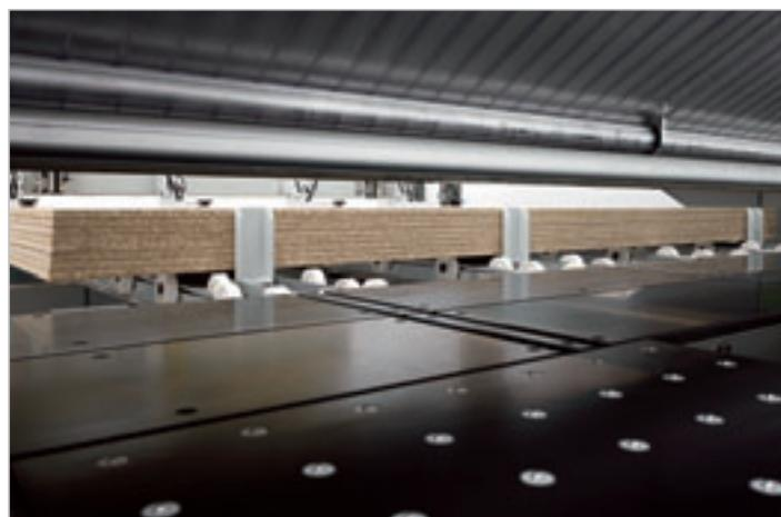
Robust front aligning devices align the stack of panels against the pusher grippers.
