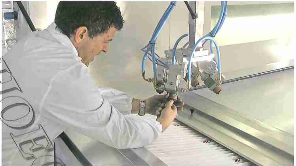
Pulizia ugelli_ Nozzle cleaning_ Reinigung der Duesen_ Nettoyage buses_ Limpieza toberas
