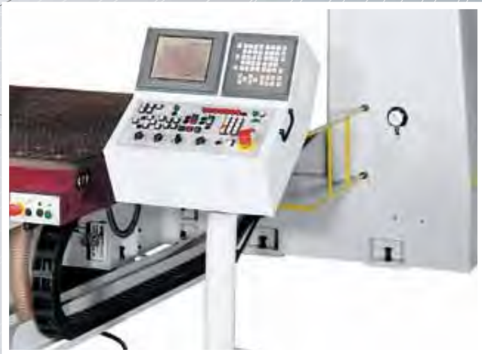
Controller options from FANUC, Syntec and Siemens allow for a wide range of motion control options.
