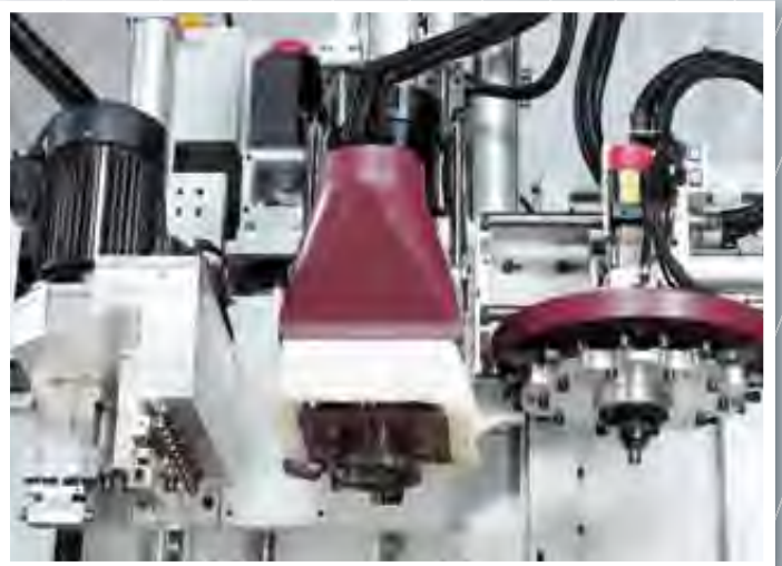
Common spindle configuration on the STRATOS Series: Line boring unit, HSK spindle, traveling tool carousel.
