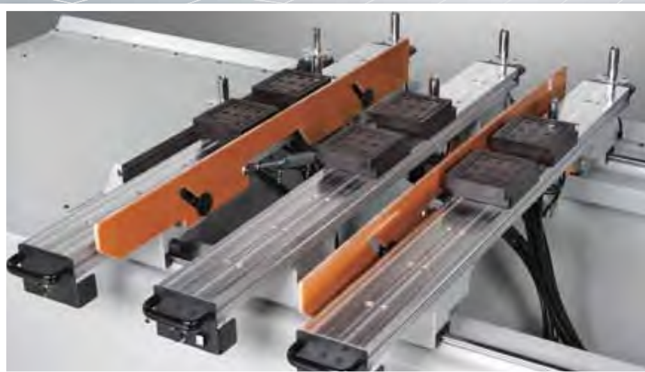
A laser positioning system is used for automatically positioning beams and suction cups. Panel lifting blades make easy work of positioning and moving heavy work pieces.
