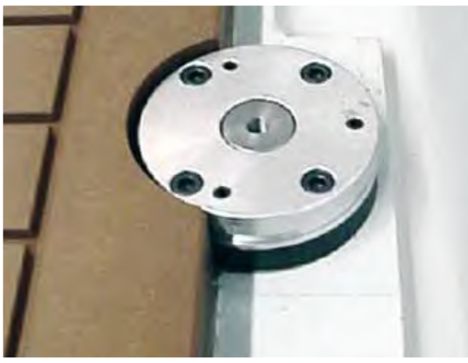
Automatic pop-up pins for assisting in part and sheet location are standard on all STRATOS Machines.
