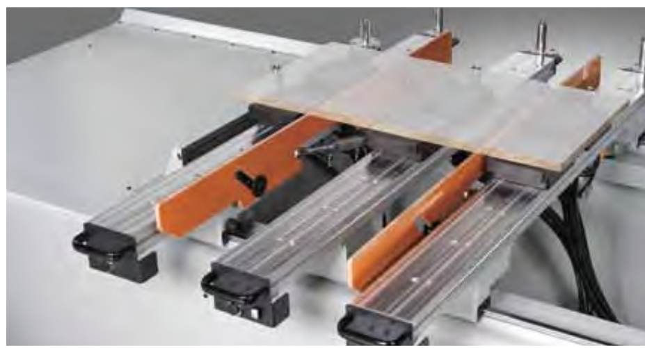
The moveable beams and suction cups allow you to process different kinds of work pieces by utilizing different manufacturing procedures.
