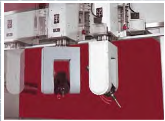
Several Spindle options are available to meet the application from 8.1 HP 40,000 rpm to 25 HP 22,000 rpm.
