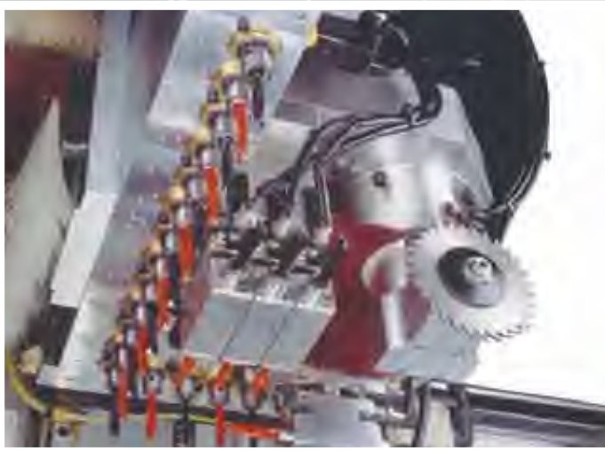
The STRATOS Series is available with multiple 32 mm system line boring units with vertical, horizontal and grooving saw options.
