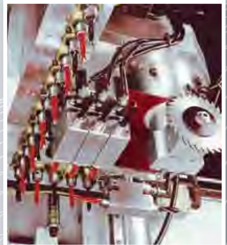
The standard 32 mm boring unit is a 10x7 vertical spindle unit with optional horizontal drills.
