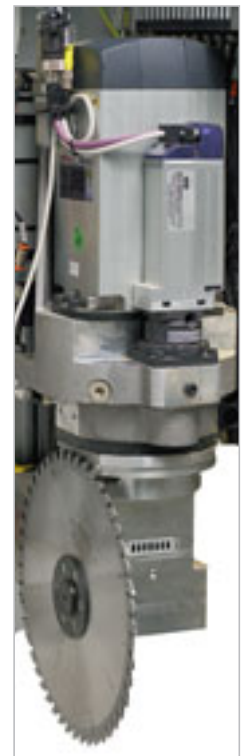
Multifunctional unit with aggregate for sawblade unit - N.C. rotation through 360°.
